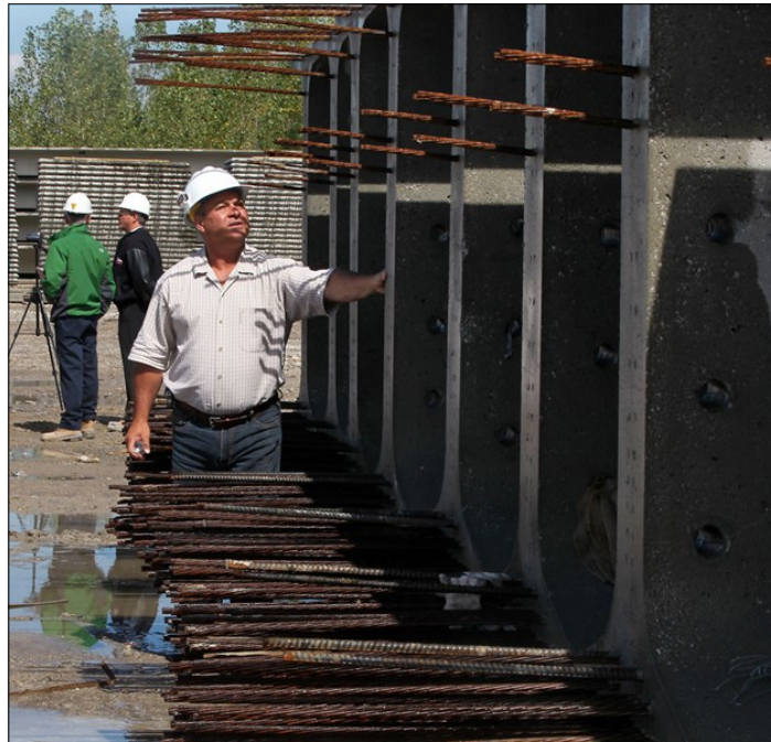
Loris Collavino, owner of Prestressed Systems Inc. inspects some of 546 concrete and steel bridge girders which will be used on The Windsor-Essex Parkway. The girders are structural members that span over the main roadway. (NICK BRANCACCIO/The Windsor Star)
